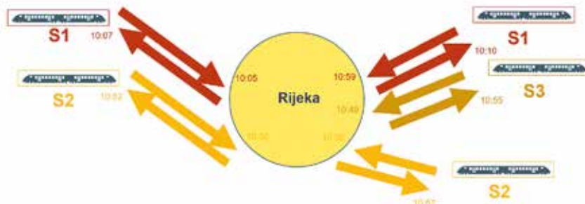
Figure 14 - Timetable diagram for Rijeka railway station for the second 30 minutes with arrivals and departures for suburban trains only. Source: made by authors
