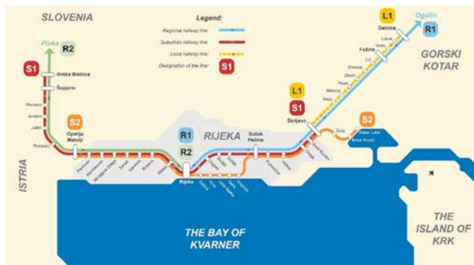
Figure 10 - Schematic map of Rijeka region suburban railway services, phase 2. Source: made by authors
