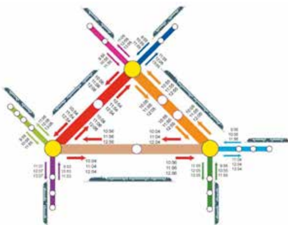
Figure 6 - Integrated clock-face timetable applied on a network with the examples of arrivals and departures of trains.
